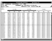
Recorded measurement data from up to 10 channels are displayed at the monitor in numeric format in an easy to read table.
